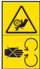
Danger rotating parts. Keep clear of moving/rotating parts in chamber.
