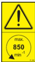
Make sure the transmission is running with the correct speed and direction. Wrong speed and/or direction can damage machinery and may cause great danger to persons nearby. The machine is designed for a PTO-speed of 850 rpm.
