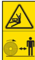
Operator or others close to the machine must be aware when the bale is unloaded from the wrapper table. Bales dropped may roll more than 10 m, or even dropped prematurely.
