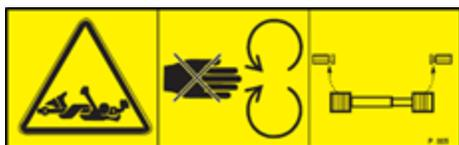
Between the tractor and the machine, there is a rotating PTO-shaft. No one is allowed to stand between the tractor and the machine while the engine is running. Do not wear loose clothes, scarfs etc.
