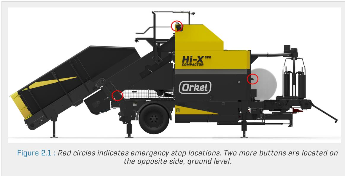
When an emergency stop button has been triggered, the emergency stop button has to be reset so that the machine can be started from the control panel.
