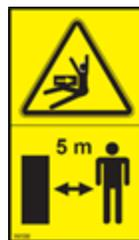
Unauthorized personell are not allowed closer than 5 meters, when the machine is operating or when maneuvering.
