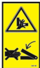
Danger. Film holder/cutter has a sharp knife and there is a risk of cutting/crushing injury. Always keep closed when the machine is not operating.
