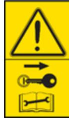
Always stop the tractor engine or external power unit before; lubricating, adjusting, maintaining or repairing the machine. Also, remove the ignition key to prevent accidental start.
