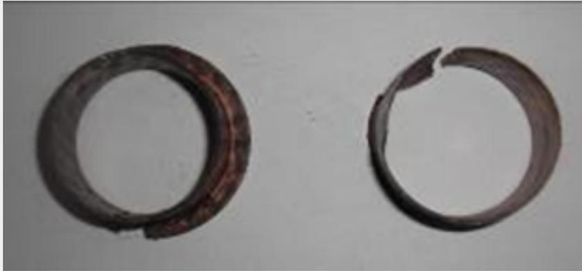
Figure 7.30 : Example picture of plain bearing. New bearing to the left, and worn out/defect bearing to the right.
