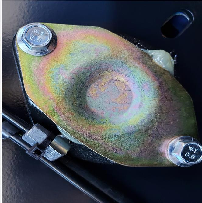
[Figure 2.3](#) : Grease collar on bearings/bushings
