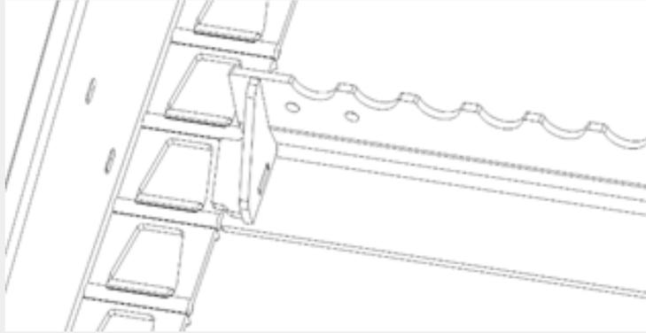
Figure 7.5 : Elevator conveyor chain
