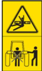
Ensure that there are no people between tractor and machine during connecting and disconnecting.
