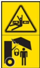
Always use the hydraulic securing valves on the chamber door lifting cylinders, to ensure that the chamber door stays in open position during maintenance or repair.
